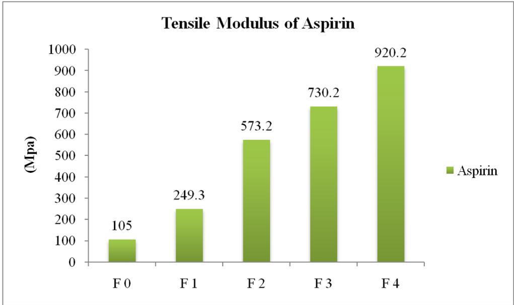
**Figure 3.** Tensile modulus of the cellulose polymer nanocomposite film containing aspirin (FA).
