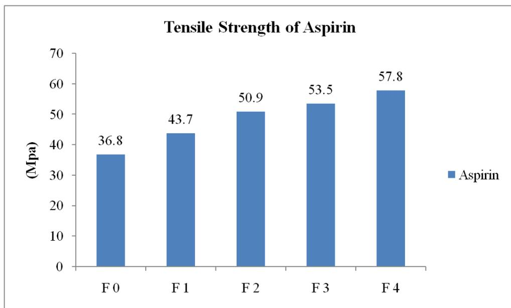
**Figure 2.** Tensile strength of the cellulose polymer nanocomposite film containing aspirin (FA).
