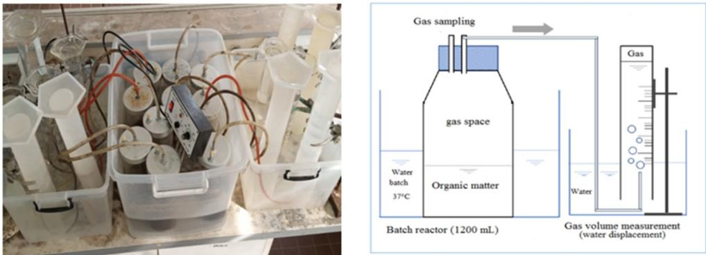
**Figure 2.** Anaerobic digestion test setup.
