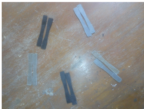
Figure 3: Samples for tensile strength test.
