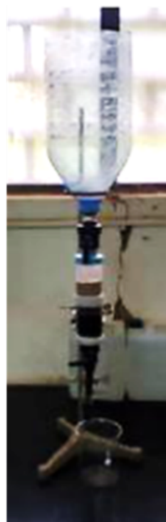
Figure 2. Double column diagram (activated carbon topped with zircon).
